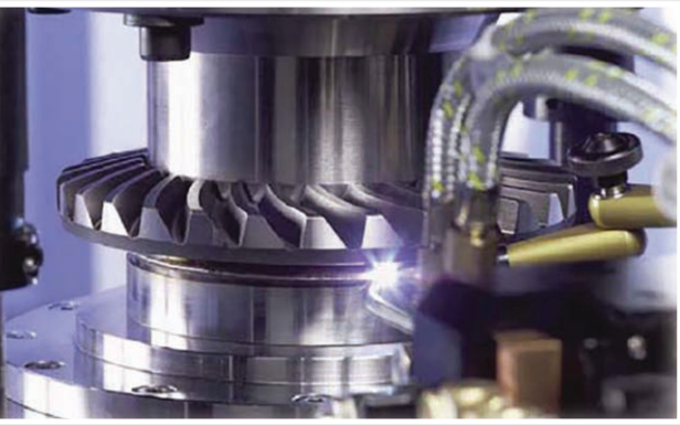
Powertrain Part welded with Laser and Filler Wire
