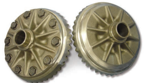
Bolted Design vs. Laser Welded Design for an Automotive Differential Unit
