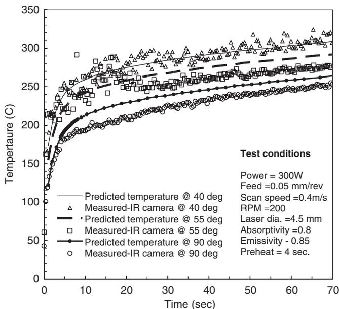
Fig. 10. Comparison of maximum predicted and measured temperature at different circumferential locations with infrared camera.
