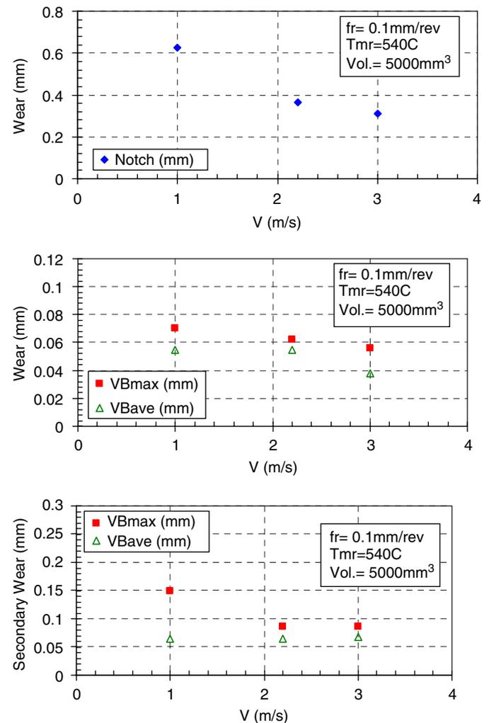
Fig. 14. (a) Notch wear, (b) primary flank wear, and (c) wear on the secondary face measured at approximately 5000 mm<sup>3</sup> of material removed (L13, L11, L14) ( $fr = 0.1$  mm/rev,  $d = 0.76$  mm,  $T_{mr,ave} = 540$  °C).
