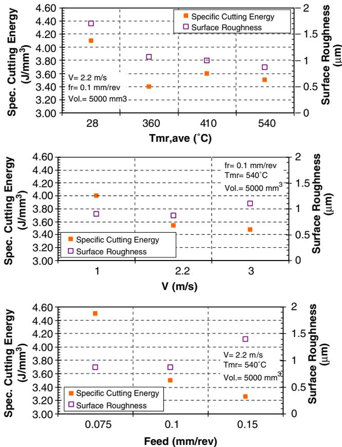
Fig. 12. Specific cutting energy and surface roughness vs.  $T_{mr,ave}$ , velocity, and feed, measured after removing 5000 mm<sup>3</sup> of material.
