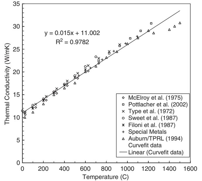
Fig. 2. Comparison of temperature-dependent thermal conductivity of Inconel 718.
