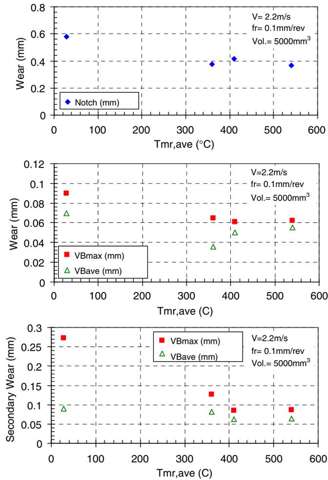
Fig. 13. (a) Notch wear, (b) primary flank wear, and (c) wear on the secondary face measured at approximately 5000 mm<sup>3</sup> of material removed (L8, L16, L17, L11) ( $V = 2.2$  m/s,  $fr = 0.1$  mm/rev,  $d = 0.76$  mm).
