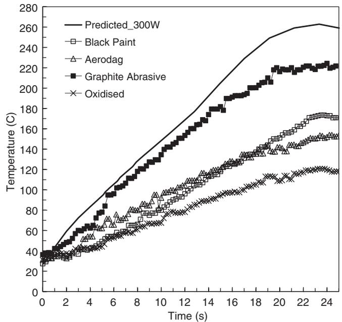
Fig. 5. Comparison of measured and predicted temperatures for power-300 W.
