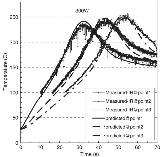
Fig. 8. Predicted and measured temperature history (300 W).
