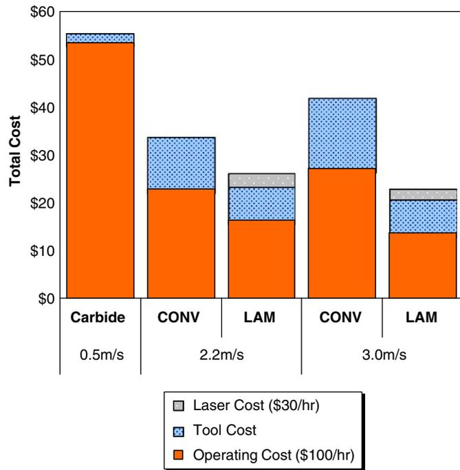
Fig. 16. Total cost comparison when machining 1 m length (or 58,000 mm<sup>3</sup>) by conventional machining and LAM.
