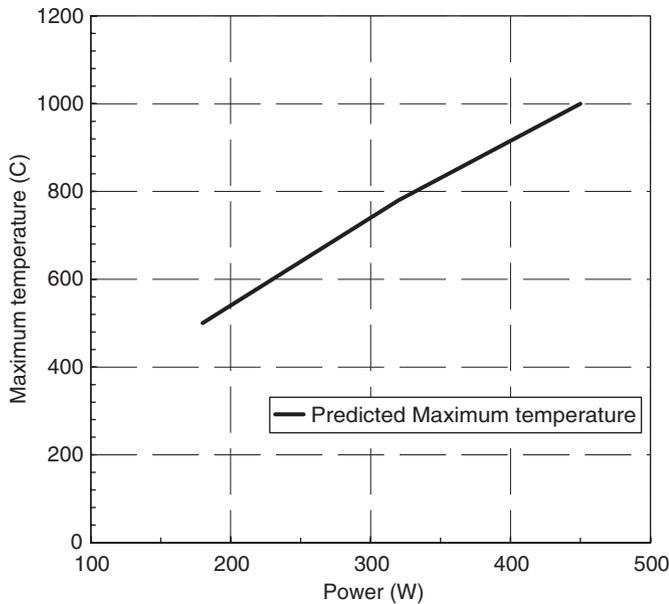
Fig. 9. Variation of maximum temperature under the laser spot with laser power.
