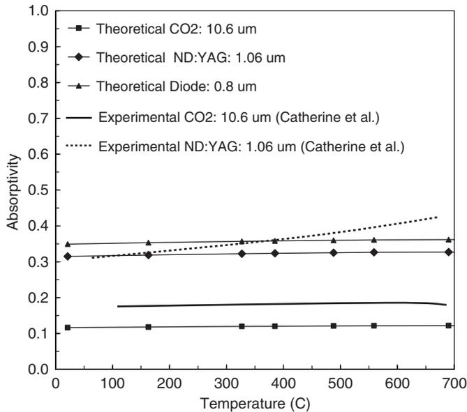
Fig. 4. Theoretical and experimental normal spectral absorptivity of Inconel 718 at different laser wavelengths.
