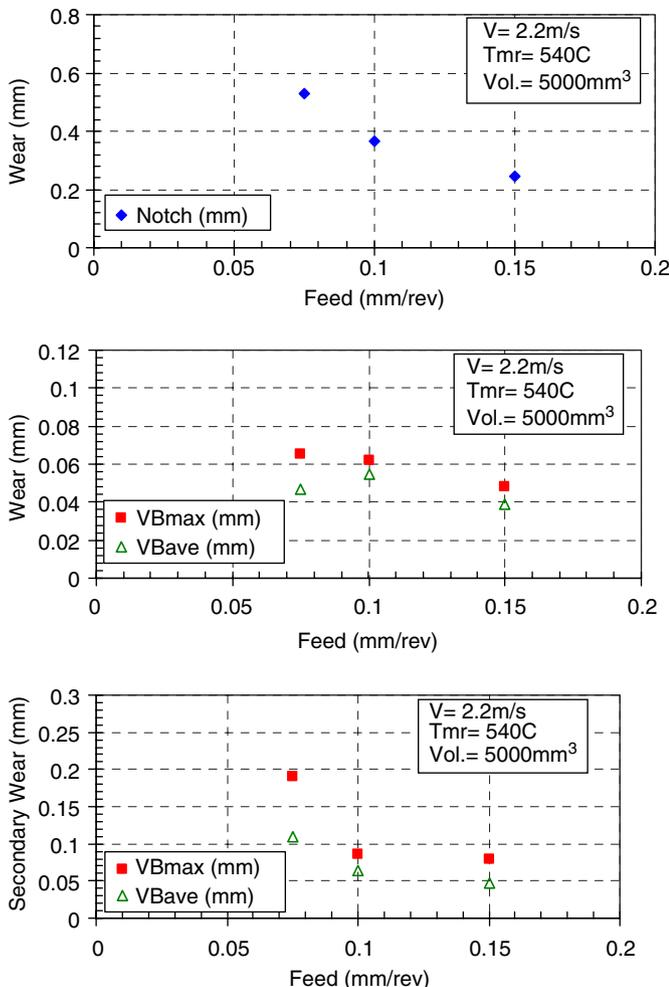
Fig. 15. (a) Notch wear, (b) primary flank wear, and (c) wear on the secondary face measured at approximately 5000 mm<sup>3</sup> of material removed (LAM7, L11, L12) ( $V = 2.2$  m/s,  $d = 0.76$  mm,  $T_{mr,ave} = 540$  °C).
