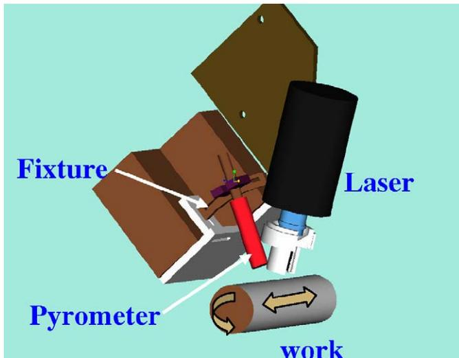
Fig. 6. Schematic illustration of in-process temperature measurement with a pyrometer.
