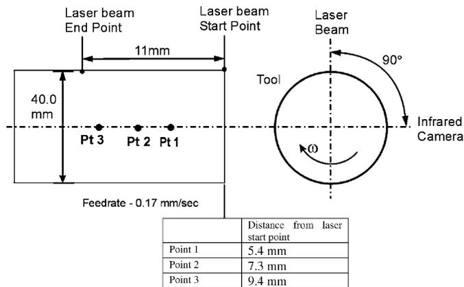
Fig. 7. Measurement locations for the infrared camera ( $\lambda = 8-9 \mu\text{m}$ ).
