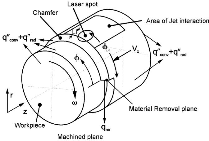
Fig. 1. Model geometry for the laser-assisted machining of a cylindrical workpiece [10].
