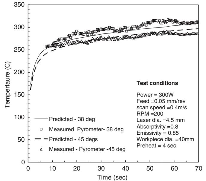
Fig. 11. Comparison of maximum predicted and measured temperature at different circumferential locations with the radiation pyrometer.
