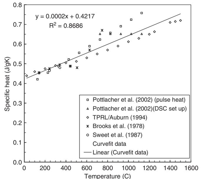
Fig. 3. Comparison of temperature-dependent specific heat of Inconel 718.
