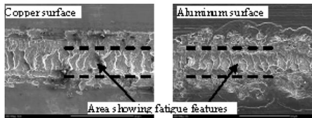
**Figure 12. SEM Pictures of Fractured Weld Interfaces after Fatigue Testing on cw Lap-Joined Al to Cu**
