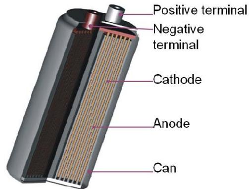
**Figure 1. Schematic Showing Different Components of a Li-Ion Cell**
