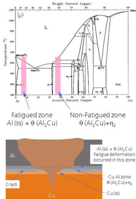
**Figure 14. Cu-Al Binary Phase Diagram Showing the Phases Corresponding to Fatigued and Non-Fatigued Zones and their Respective Elemental Composition (top) - The Schematic Shows the Proposed Mechanism for Crack Propagation (bottom)**
