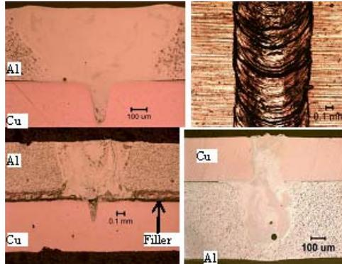
**Figure 9. Top view and Cross-Sections of cw Overlap Joints of Al and Cu**
