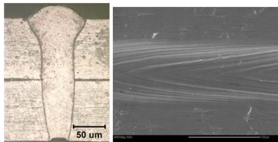
**Figure 1. Overlap Penetration Weld at 50 m/min in Stainless Steel**
