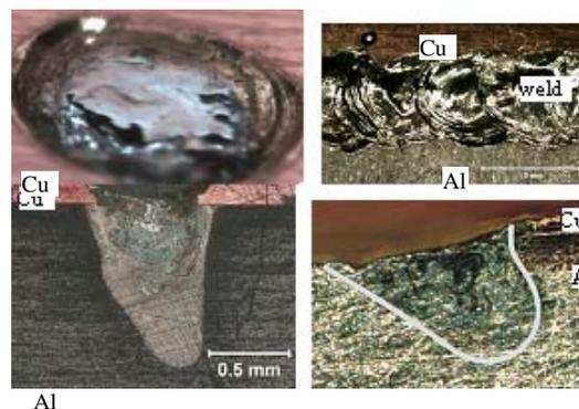
**Figure 8. Top Views and Cross-Sections of Pulsed Lap (left) and Pulsed Edge (right) Welds of Cu to Al**
