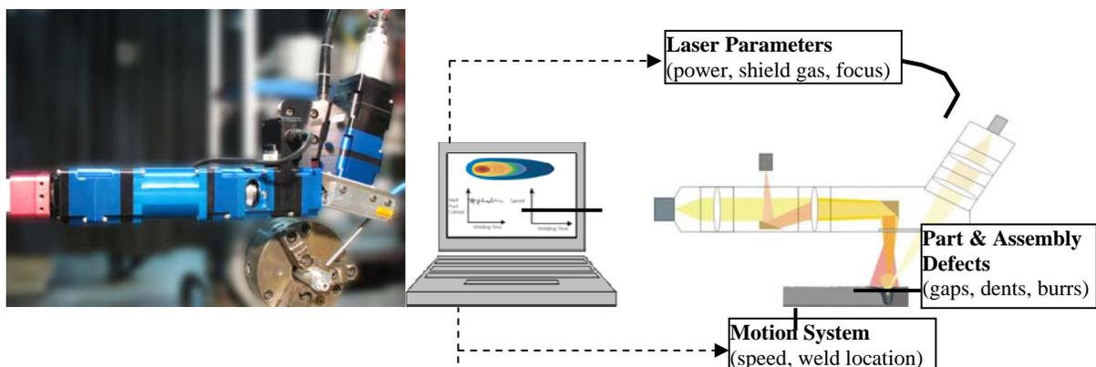
**Figure 15. Component Diagram (right) for Coaxial Process Monitoring Setup** [Actual (left) setup used for highly reflective metal welding.]
