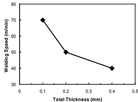
**Figure 2. Maximum Welding Speed in Dependency of Material Thickness**
