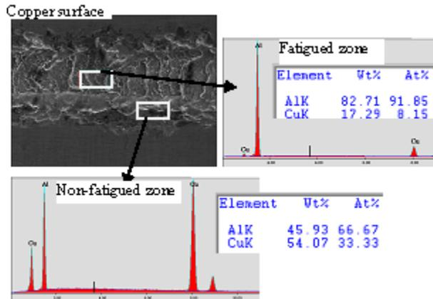
**Figure 13. TEM Analysis of Fractured Weld Interfaces after Fatigue Testing on cw Lap-Joined Al on Cu**
