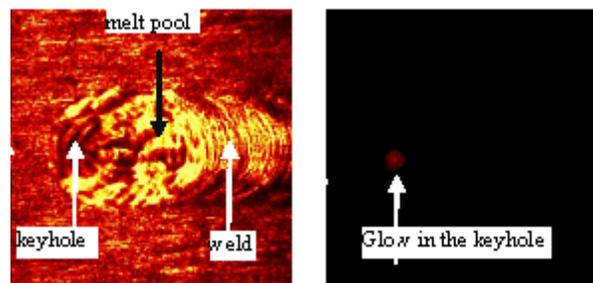
**Figure 16. High-Speed Camera Pictures of Welding Process Showing the Melt Pool with (left) and without (right) Coaxial Illumination.**
