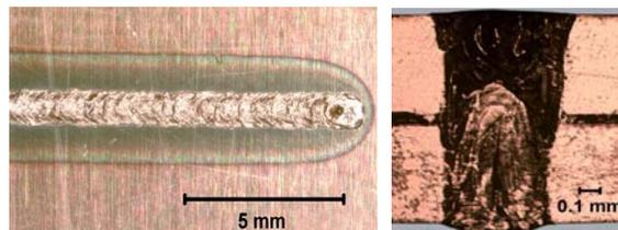
**Figure 2. Top and Cross-Section View of Cu for Overlap Welding using a Multi-Mode (MM) Fiber Laser**
