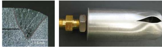
**Figure 4. Cross Section of Welded Joint (left) - Failed Al Can after Burst Test**
