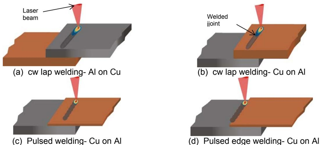
**Figure 7. Different Joint Configurations for Welding Al to Cu**
