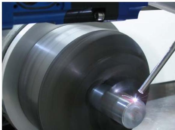
**Figure 3. Laser Welding of Al Lid to Can**
