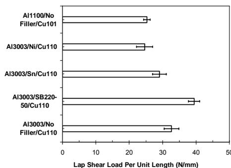
**Figure 10. Maximum Lap Shear Load per Unit Length for Different Combinations of Base and Filler Material for cw Lap Joining of Al on Cu**
