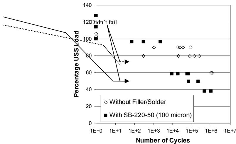
**Figure 11. Fatigue Strength for cw Lap Joining of Al on Cu-Welded with and without the Filler Material**
