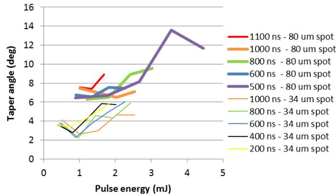
Figure 6. Taper angle versus pulse energy for 190  $\mu\text{m}$  thick wafer at different PL and spot size
