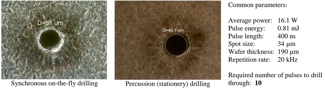
Figure 3. Drilling results from synchronous on-the-fly drilling and percussion drilling along with process parameters
