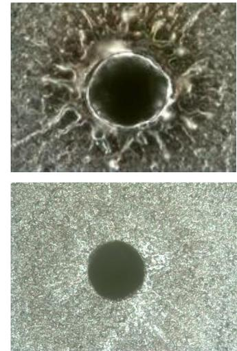
Figure 5. High (upper) and low (lower) melt spatter and recast attached to drilled hole entrance for different process parameters
