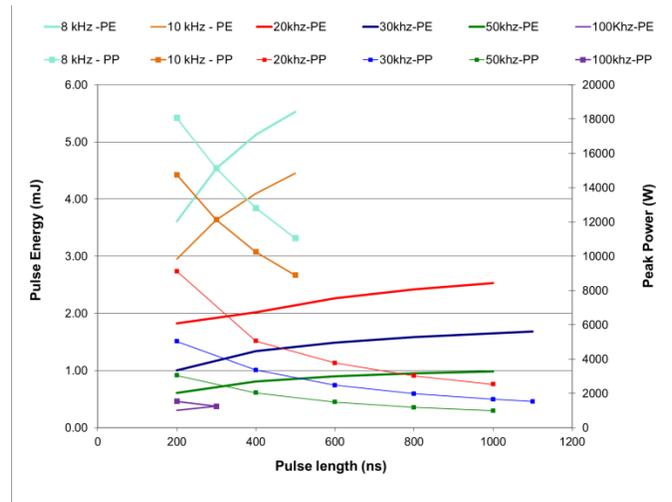
Figure 2. Power and energy characteristics of disc laser
