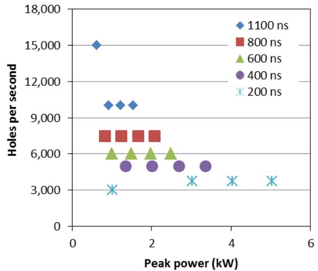
Figure 9. Drilling rate (holes/sec) versus peak power for 120 μm thick wafer
