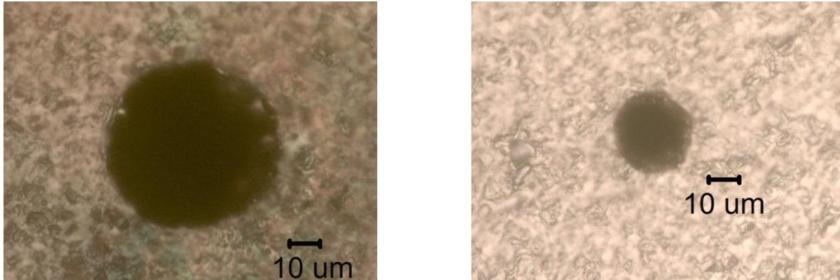
Figure 10 Hole entrance (left) and exit (right) at drill rate of 15,000 holes/sec
