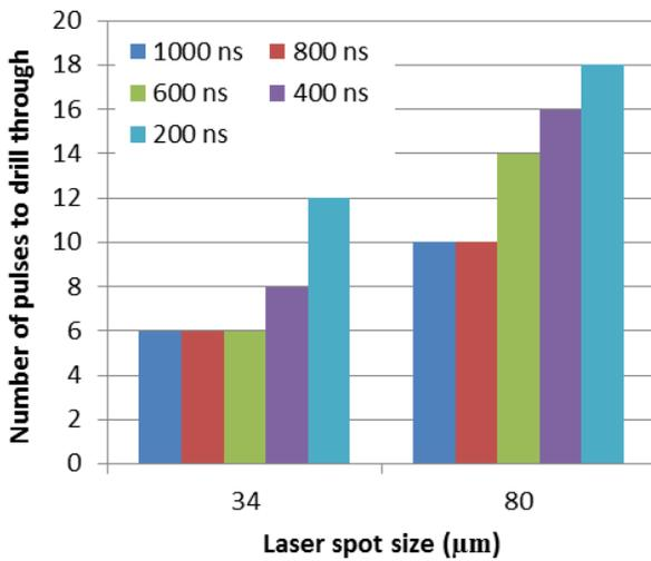
Figure 8. Number of laser pulses to drill through the wafer versus laser spot size for 190 μm thick wafer
