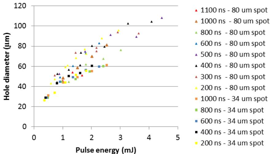
Figure 4. Average hole diameter versus pulse energy for 190  $\mu\text{m}$  thick wafer at different PL and spot size
