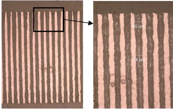
Figure 11 Cross-section of 2 mm Ta with  $105 \mu\text{m}$  spacing and post chemical etching
