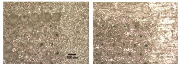
Figure 5 Surface of drilled holes ‘as is’ (left) and surface after the debris was removed using a sharp knife (right)
