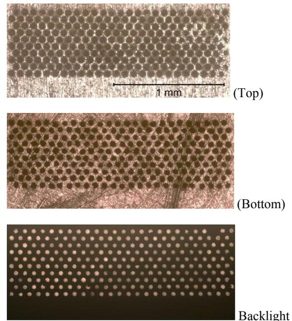
Figure 10 Array of drilled hole with entrance side (top), exit side (middle) and with backlight (bottom).
