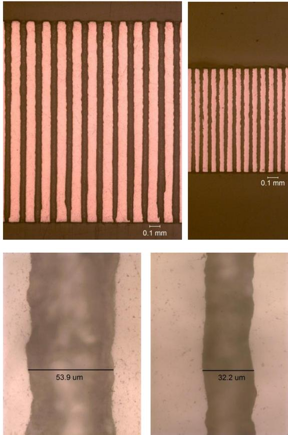
Figure 9 Best achieved drilling result in 2 mm Ta (left) and 1 mm Ta (right). The close-up of holes show diameter of  $\sim 54 \mu\text{m}$  in 2 mm (left) and  $\sim 32 \mu\text{m}$  in 1 mm (right).
