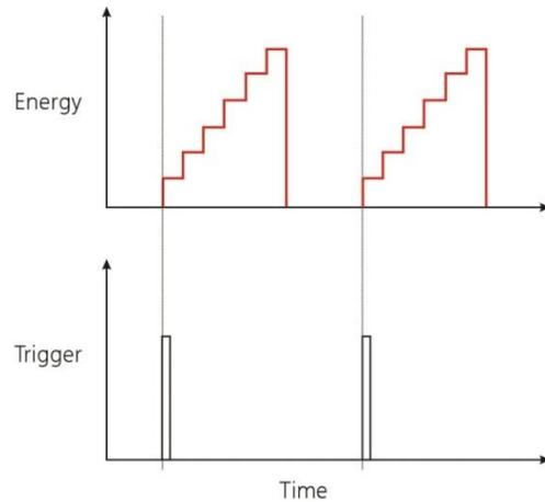
Figure 4 Schematic representation of inter-pulse shaping
