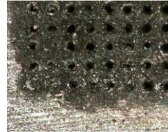
Figure 7 Drilled surface with shortest drill time of 200 ms shows significant debris even after etching for 20 min
