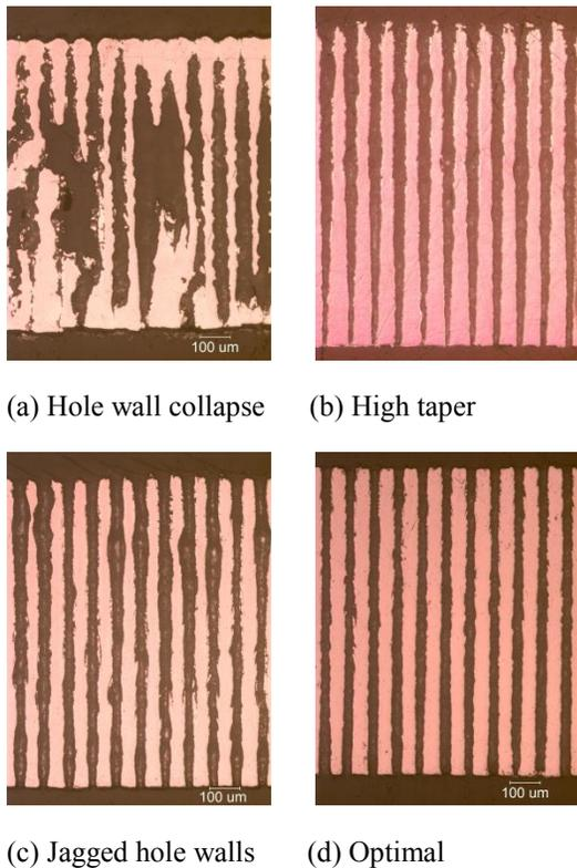
Figure 3 Hole cross-section corresponding to data points in Fig 2.
