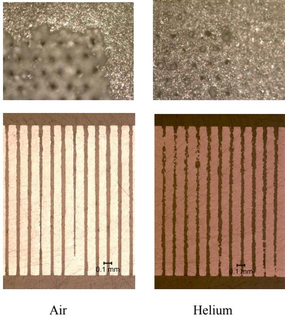
Figure 6 Drilled surface (top) and cross-section (bottom) with air (left) and helium (right)
