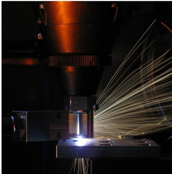
Figure 1 Laser drilling of Tantalum
