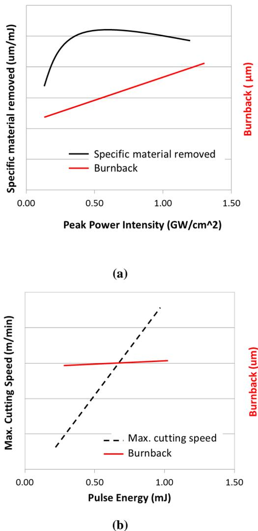
Figure 3 Process charts for pulsed cutting with IR lasers. (a) SMR and burnback versus PPI, (b) Max cutting speed and burnback versus pulse energy
