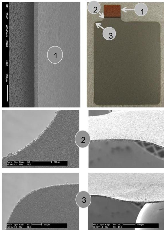
Figure 6 Remote cut prismatic cell electrode
