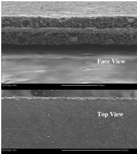
Figure 4 Pulsed IR laser cut edge of anode
