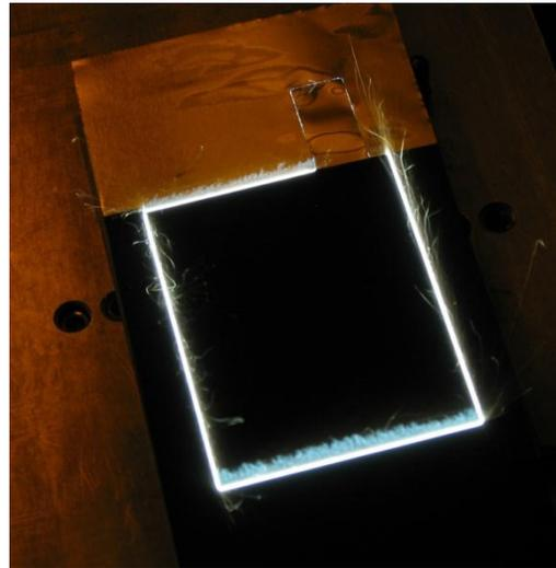
Figure 1 Laser cutting of electrode
