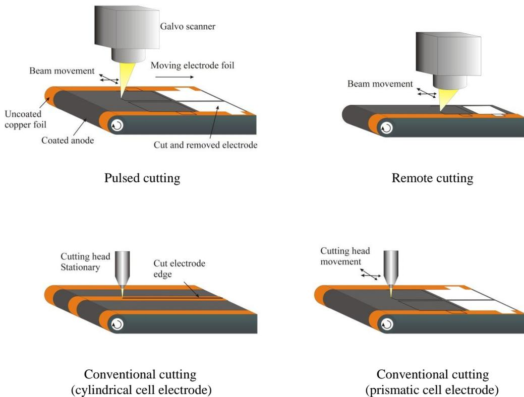
Figure 2 Schematic illustration of different laser cutting strategies
