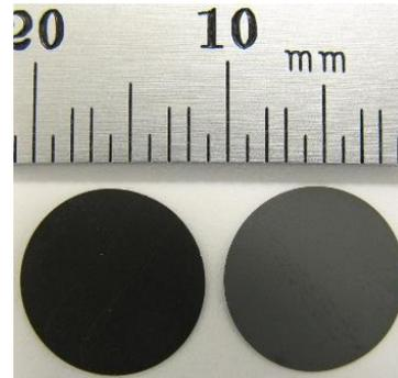
Figure 5 Pulsed UV laser cut button cell electrodes
