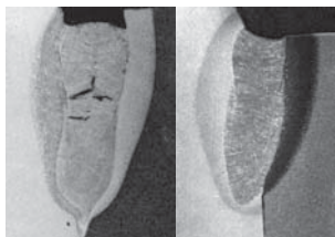
Laser Weld Joint without Induction (left) and with Induction (right)
