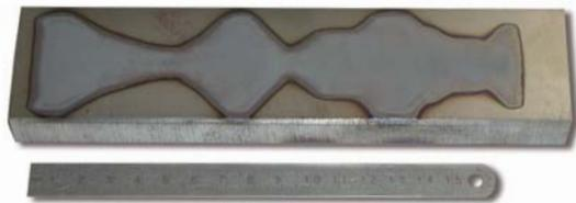
Laser Hardening with Variable Track Width
