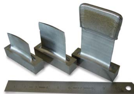
Turbine Blades repaired with Laser
