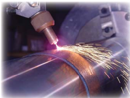
Laser Cladding Process with Cyclone Nozzle (side-axis feed design)
