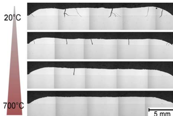
Increasing the Clad Quality of Crack Sensitive Materials with Induction Assisted Laser Cladding
