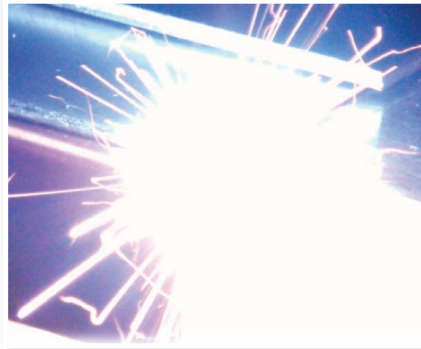
Laser Welding of Copper and Aluminum
