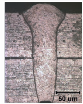
Weld Section Produced on Stainless Steel at 50 m/min
