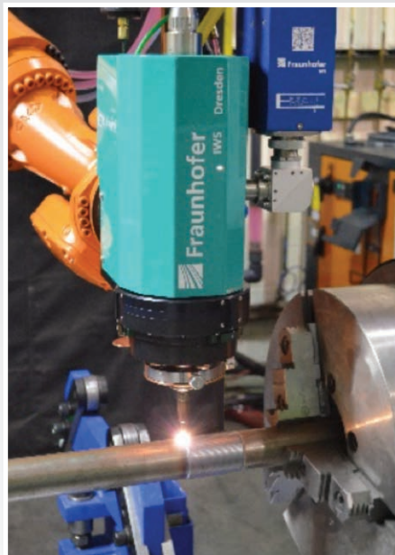
Fraunhofer IWS Coax Wire Head with EMAQS Camera mounted for coaxial process viewing and melt pool size control
