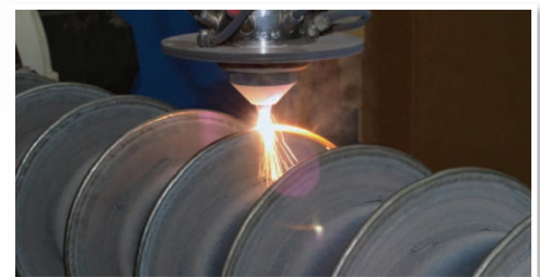
Screw Thread Build up using COAX Powder Technology
