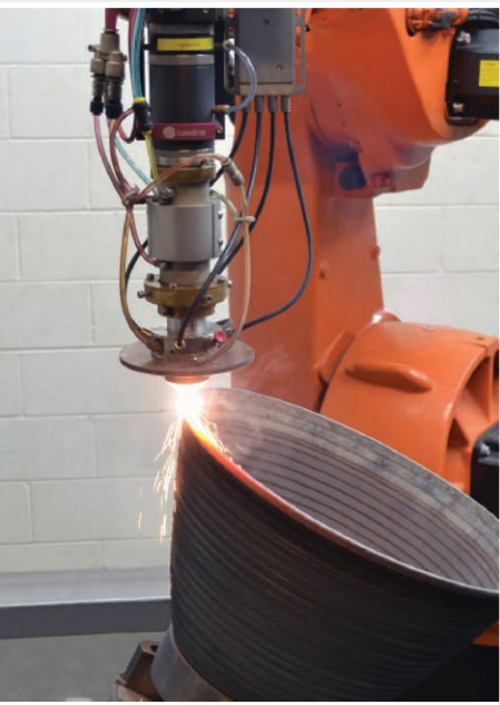
Laser Additive Manufacturing of an Aerospace Nozzle Demonstration Component
